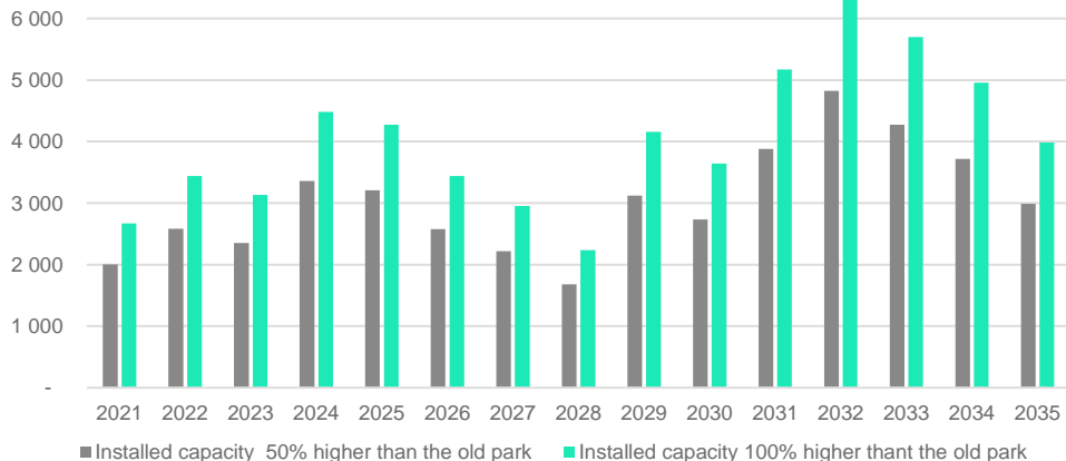
Investment in repowering each year (M €) according to the installed capacity in France
